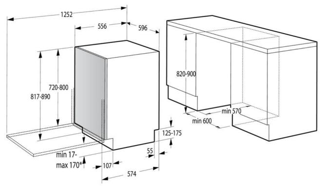
\*Because of height adjustable screw feet: Base height when appilance height is 817: 17-97 mm Base height when appliance height is 890: 90-170 mm
